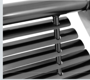
Angled louvers provide shade and protect rear window
